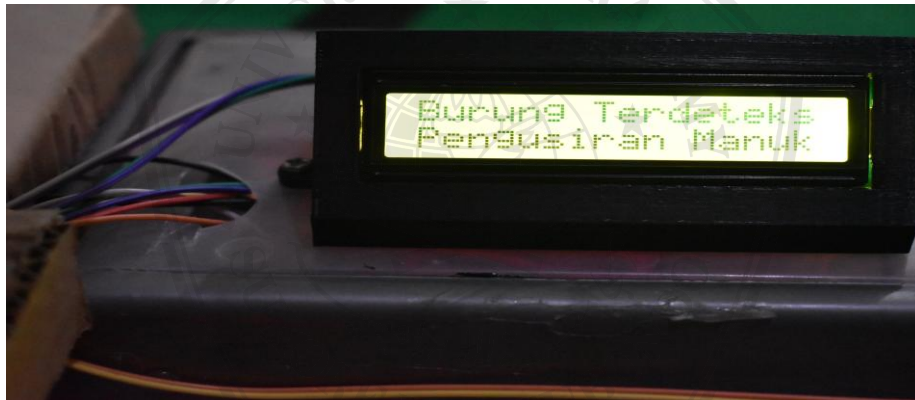
Gambar 4. 7 Status Sensor Pir
